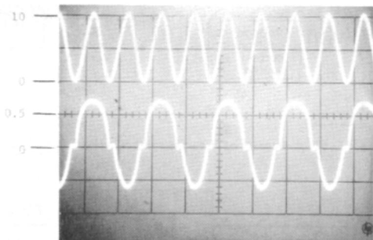
Fig. 3. Upper trace:  $V_i(t)$ , 5 V/div. Bottom trace:  $V_{out}(t)$ , 0.5 V/div.
