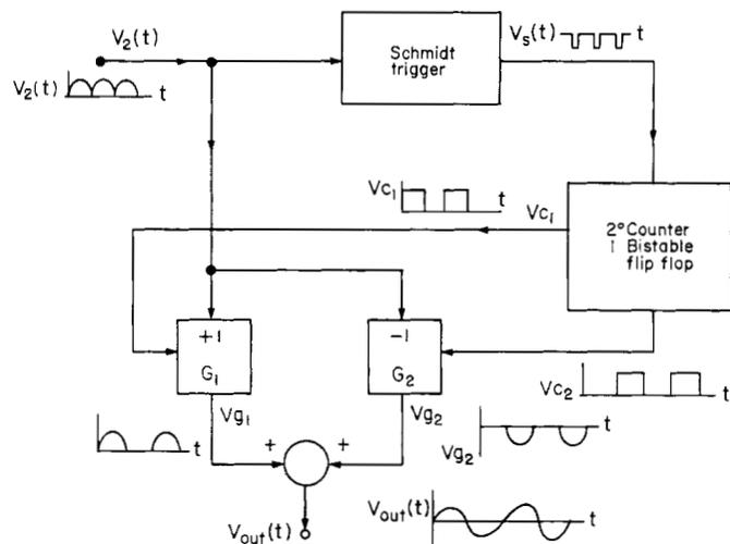
Fig. 2. Block diagram of synchronizer to generate  $V_{out}(t)$ .
