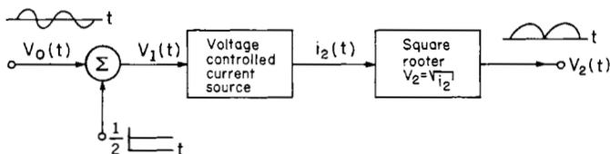
Fig. 1. Block diagram of circuit to synthesize  $V_2(t)$  from  $V_0(t)$ .
