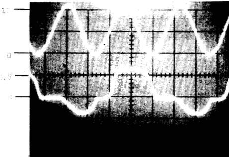
Fig. 4. Upper trace:  $V_i(t)$ , 5 V/div. Bottom trace:  $V_{out}(t)$ , 0.5 V/div. Time base: 20  $\mu$ s/div. Input frequency: 20 kHz.
