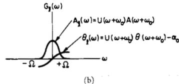
Fig. 1. (a) Symmetrical bandpass filter. (b) Low-pass equivalent filter.
