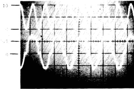
Fig. 3. Upper trace:  $V_i(t)$ , 5 V/div. Bottom trace:  $V_{out}(t)$ , 0.5 V/div. Time base: 2 ms/div. Input frequency: 500 Hz.
